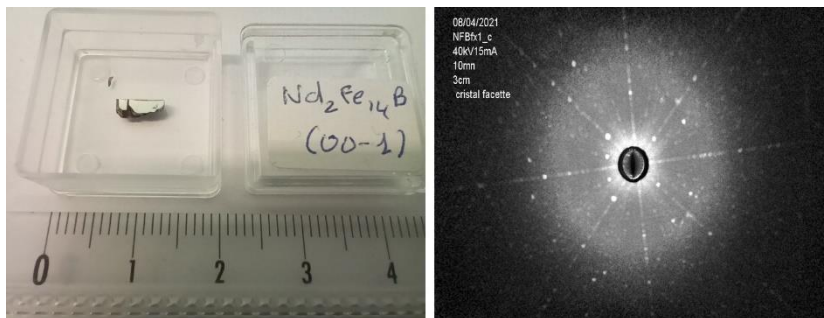
Figure: Single crystal of the Nd 2 Fe 14 B obtained by a flux method and corresponding Laue diffraction pattern.
